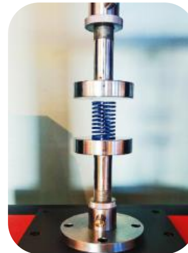
Compression Testing For Spring
