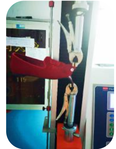
Tear Strength Testing For Leather or Fabric
