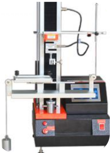
90° Peel Testing For Adhesive Tape
