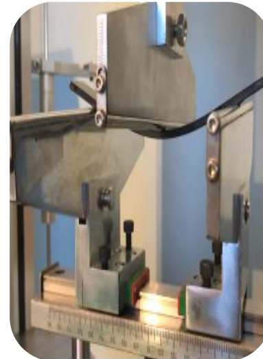
3 Point Bending Testing For Pills or other
