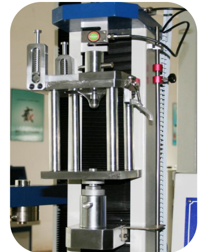
Film Puncture Testing For Film
